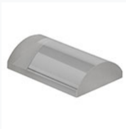
LJ4426-A: f=25.0 mm, UVFS Plano-Convex Cylindrical Lens, L=30 mm, H=20 mm, ARC: 350 - 700 nm
