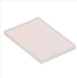
LK4989-B: f=-500.0 mm, Plano-Concave Cylindrical Lens, UV Grade Fused Silica, H=30.0 mm, L=45.0 mm, ARC: 650 - 1050 nm
