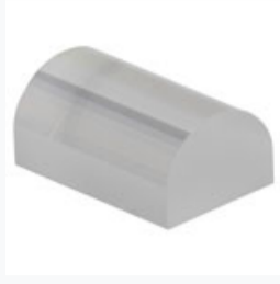
LJ4359-C: f=8.0 mm, UVFS Plano-Convex Cylindrical Lens, L=11 mm, H=7.2 mm, ARC: 1050 - 1700 nm
