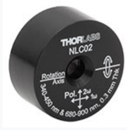
NLC02: Ø1" Mounted \beta -BBO Crystal, 0.30 mm Thick, \theta = 30.5^\circ , 680 - 900 nm Fund., 340 - 450 nm SHG
