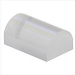
LJ4359-B: f=8.0 mm, UVFS Plano-Convex Cylindrical Lens, L=11 mm, H=7.2 mm, ARC: 650 - 1050 nm
