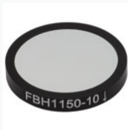
FBH1150-10: Premium Bandpass Filter, Ø25 mm, CWL = 1150 nm, FWHM = 10 nm
