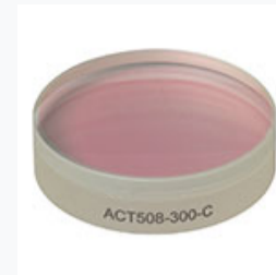
ACT508-300-C: f = 300.0 mm, Ø2" Achromatic Doublet, ARC: 1050 - 1700 nm
