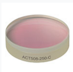
ACT508-250-C: f = 250.0 mm, Ø2" Achromatic Doublet, ARC: 1050 - 1700 nm
