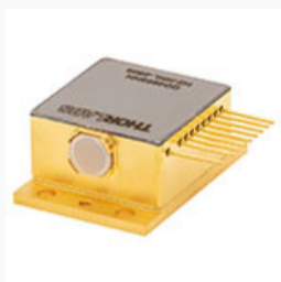
QD4602HH: DFB QCL, 4.602 \mu\text{m} CWL, 3 \text{cm}^{-1} Tuning, 30 mW, Horizontal HHL
