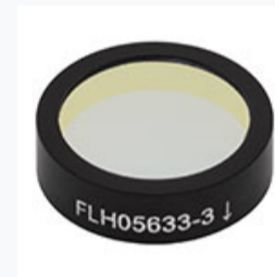
FLH05633-3: Premium Bandpass Filter, Ø12.5 mm, CWL = 632.8 nm, FWHM = 3 nm
