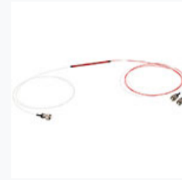
PNH1310R1F1: 1x2 PM Coupler, 1310 \pm 15 nm, 99:1 Split, \geq 25 dB PER, FC/PC Connectors
