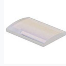
LJ4395-B: f=100.0 mm, UVFS Plano-Convex Cylindrical Lens, L=45 mm, H=30 mm, ARC: 650 - 1050 nm
