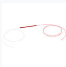
TG625R2B1A: 1x2 MM Dual-Window Fiber Coupler, Ø62.5 Core, 0.275 NA, 90:10 Split, No Connectors
