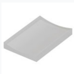
LK4245-C: f=-100.0 mm, Plano-Concave Cylindrical Lens, UV Grade Fused Silica, H=30.0 mm, L=45.0 mm, ARC: 1050 - 1700 nm
