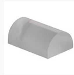
LJ4918-A: f=10.0 mm, UVFS Plano-Convex Cylindrical Lens, L=14 mm, H=9 mm, ARC: 350 - 700 nm
