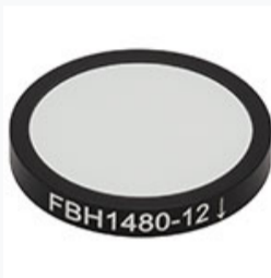
FBH1480-12: Premium Bandpass Filter, Ø25 mm, CWL = 1480 nm, FWHM = 12 nm
