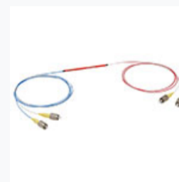
TW2000R2F2C: 2x2 Wideband Fiber Optic Coupler, 2000 \pm 150 nm, 90:10 Split, SM1950 Fiber, FC/PC
