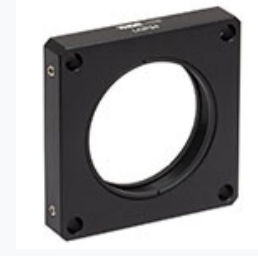
LCP34: 60 mm Cage Plate, SM2 Threads, 0.5" Thick, 8-32 Tap (Two SM2RR Retaining Rings Included)
