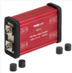
BXP13: 2x2 Boxed PM Fiber Coupler, 1550 ± 15 nm, 75:25 Split, ≥20 dB PER, FC/APC Bulkheads
