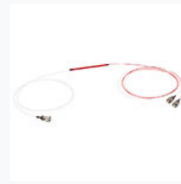
PW1550R1F1: 1x2 Wideband PM Coupler, 1550 ± 100 nm, 99:1 Split, ≥ 18 dB PER, FC/PC Connectors
