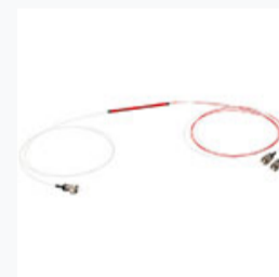
PNH1310R2F1: 1x2 PM Coupler, 1310 \pm 15 nm, 90:10 Split, \geq 25 dB PER, FC/PC Connectors
