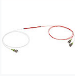
PNH1310R2A1: 1x2 PM Coupler, 1310 ± 15 nm, 90:10 Split, ≥25 dB PER, FC/APC Connectors
