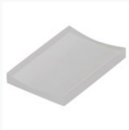
LK4385-C: f=-75.0 mm, Plano-Concave Cylindrical Lens, UV Grade Fused Silica, H=20.0 mm, L=30.0 mm, ARC: 1050 - 1700 nm
