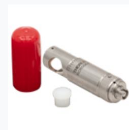
RCR50A-P01: Protected Silver Compact Reflective Collimator, 450 nm - 20 µm, RFL = 50.8 mm, FC/APC
