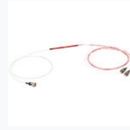
PNH1310R3F1: 1x2 PM Coupler, 1310 ± 15 nm, 75:25 Split, ≥25 dB PER, FC/PC Connectors
