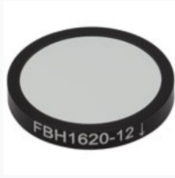
FBH1620-12: Premium Bandpass Filter, Ø25 mm, CWL = 1620 nm, FWHM = 12 nm
