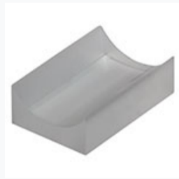
LK4155-A: f=-12.7 mm, Plano-Concave Cylindrical Lens, UV Grade Fused Silica, H=10.0 mm, L=15.0 mm, ARC: 350 - 700 nm
