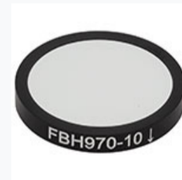
FBH970-10: Premium Bandpass Filter, Ø25 mm, CWL = 970 nm, FWHM = 10 nm
