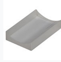
LK4326-A: f=-25.0 mm, Plano-Concave Cylindrical Lens, UV Grade Fused Silica, H=15.0 mm, L=23.0 mm, ARC: 350 - 700 nm
