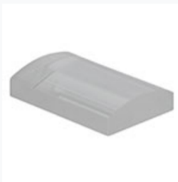
LJ4794-A: f=25.0 mm, UVFS Plano-Convex Cylindrical Lens, L=15 mm, H=10 mm, ARC: 350 - 700 nm
