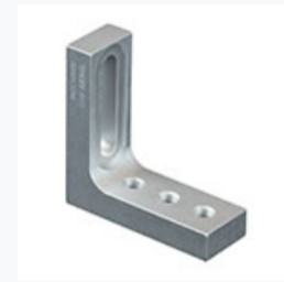
AB90CV/M: Vacuum-Compatible Slim Right-Angle Bracket with Counterbored Slot & M6 Tapped Holes
