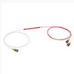
PW1550R3A1: 1x2 Wideband PM Coupler, 1550 ± 100 nm, 75:25 Split, ≥18 dB PER, FC/APC Connectors
