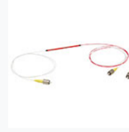
TW2000R3F1C: 1x2 Wideband Fiber Optic Coupler, 2000 ± 150 nm, 75:25 Split, SM1950 Fiber, FC/PC
