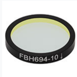
FBH694-10: Premium Bandpass Filter, Ø25 mm, CWL = 694 nm, FWHM = 10 nm
