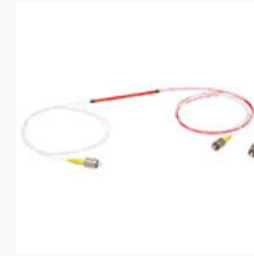
TW2000R5F1C: 1x2 Wideband Fiber Optic Coupler, 2000 ± 150 nm, 50:50 Split, SM1950 Fiber, FC/PC
