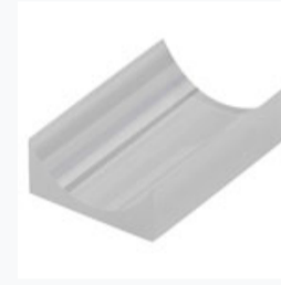
LK4498-C: f=-25.4 mm, Plano-Concave Cylindrical Lens, UV Grade Fused Silica, H=22.0 mm, L=33.0 mm, ARC: 1050 - 1700 nm
