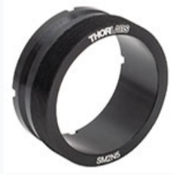
SM2N5: Nikon Eclipse Ti2 Microscope Epi-Illumination Module Adapter, External SM2 Threads
