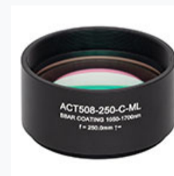
ACT508-250-C-ML: f=250 mm, Ø2" Achromatic Doublet, SM2-Threaded Mount, ARC: 1050-1700 nm
