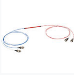
PNH1310R3F2: 2x2 PM Coupler, 1310 \pm 15 nm, 75:25 Split, \geq 25 dB PER, FC/PC Connectors
