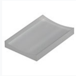
LK4245-A: f=-100.0 mm, Plano-Concave Cylindrical Lens, UV Grade Fused Silica, H=30.0 mm, L=45.0 mm, ARC: 350 - 700 nm
