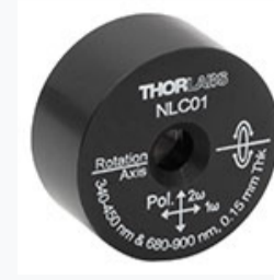
NLC01: Ø1" Mounted \beta -BBO Crystal, 0.15 mm Thick, \theta = 30.5^\circ , 680 - 900 nm Fund., 340 - 450 nm SHG
