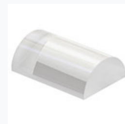
LJ4107-B: f=25.4 mm, UVFS Plano-Convex Cylindrical Lens, L=35 mm, H=23 mm, ARC: 650 - 1050 nm
