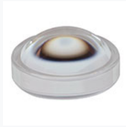
Copyright © 1999-2025 THORLABS, INC. 357610-A: f = 4.0 mm, NA = 0.6 , WD = 1.5 mm, Unmounted Aspheric Lens, ARC: 350
