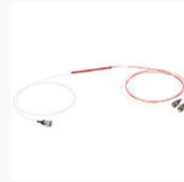
PNH1310R5F1: 1x2 PM Coupler, 1310 ± 15 nm, 50:50 Split, ≥25 dB PER, FC/PC Connectors
