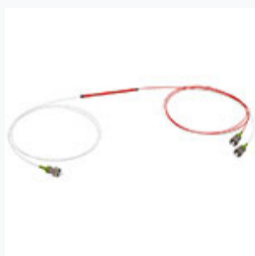
PNH1310R1A1: 1x2 PM Coupler, 1310 \pm 15 nm, 99:1 Split, \geq 25 dB PER, FC/APC Connectors
