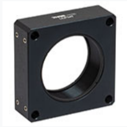
LCP34T: 60 mm Cage Plate, SM2 Threads, 0.9" Thick, 8-32 Tap (Two SM2RR Retaining Rings Included)
