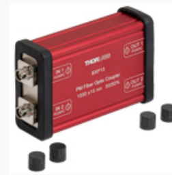
BXP15: 2x2 Boxed PM Fiber Coupler, 1550 ± 15 nm, 50:50 Split, ≥20 dB PER, FC/APC Bulkheads
