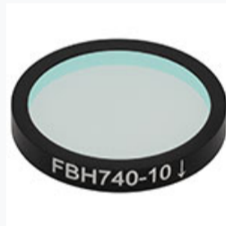
FBH740-10: Premium Bandpass Filter, Ø25 mm, CWL = 740 nm, FWHM = 10 nm
